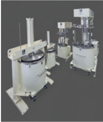
Figure 2. Change-can dual-shaft mixers with discharge systems are widely used for processing glue stick hot melts, pressure-sensitive adhesives, RTV silicon compounds and many other formulations under 500,000 cP. The use of a discharge system eliminates hours of scraping heavy or sticky materials from a mix vessel. With push-button simplicity, the system can automatically discharge several hundred gallons of product in minutes.
