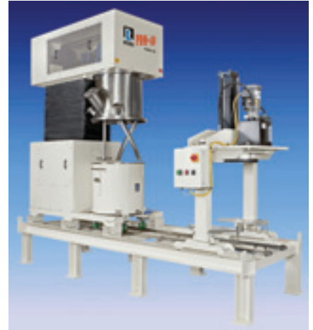
Figure 3. 40-gal planetary disperser on a raised base. After the mixing cycle, the vessel is rolled over to the discharge station. A precisely machined platen is lowered hydraulically into the vessel, forcing the finished product out of the bottom valve. The raised base allows for product to be discharged directly into 5-gal pails positioned underneath the vessel.
